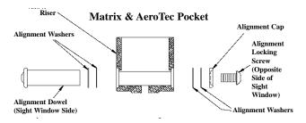
3. To reassemble the pocket, first insert the alignment dowel and washers in the riser (be sure to always put the alignment dowel in on the sight window side of the riser). Place the washers, alignment cap and alignment locking screw in the dowel. Be sure washers are not caught on the threads of the alignment screw, they must be flat against dowel shoulder prior to tightening.
